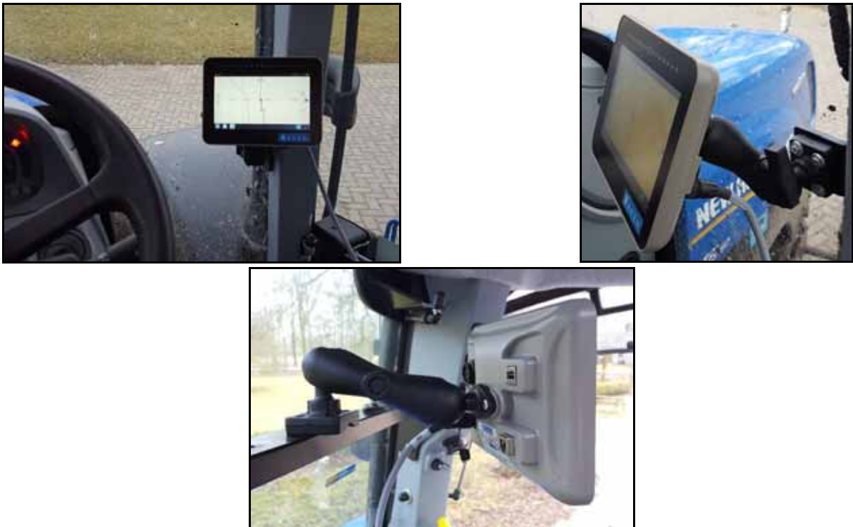
FIGURE 17. CR12 Mounted in Various Positions
