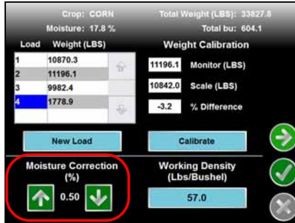
3. Touch the up or down arrows displayed in the lower, left corner of the weight calibration screen to increase or decrease the moisture correction percent in increments of 0.25%.
