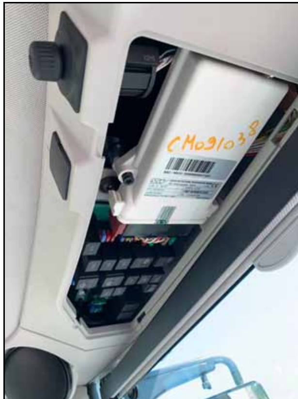
FIGURE 1. AGCO Guidance Controller Ceiling Mount Location
