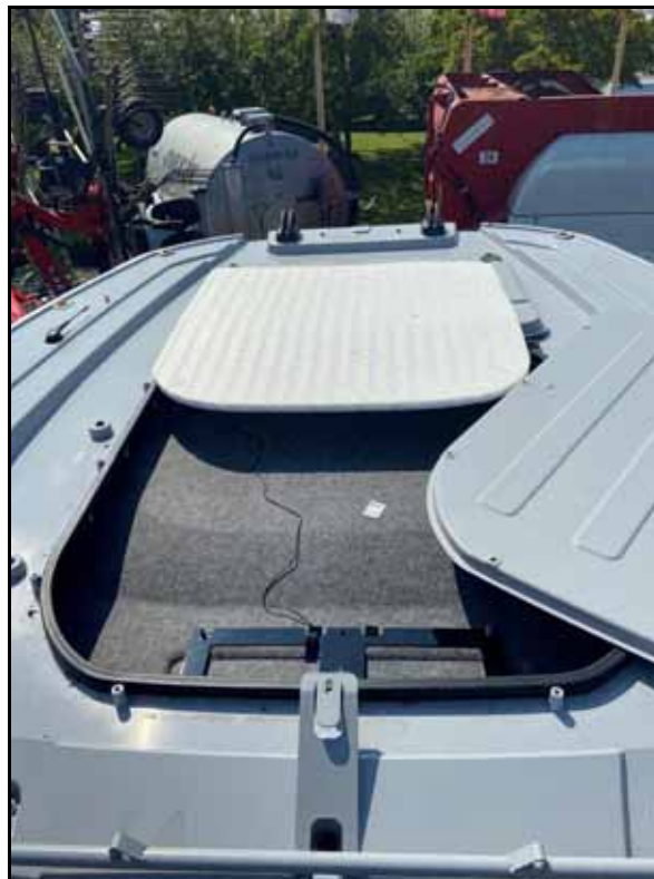
FIGURE 8. Roof Access Panel and Insulation Removed
