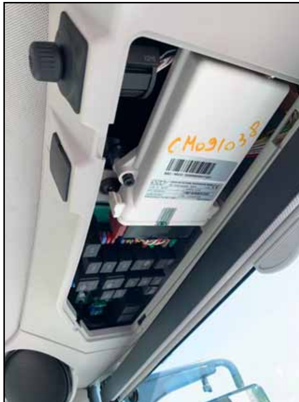
FIGURE 1. AGCO Guidance Controller Ceiling Mount Location
