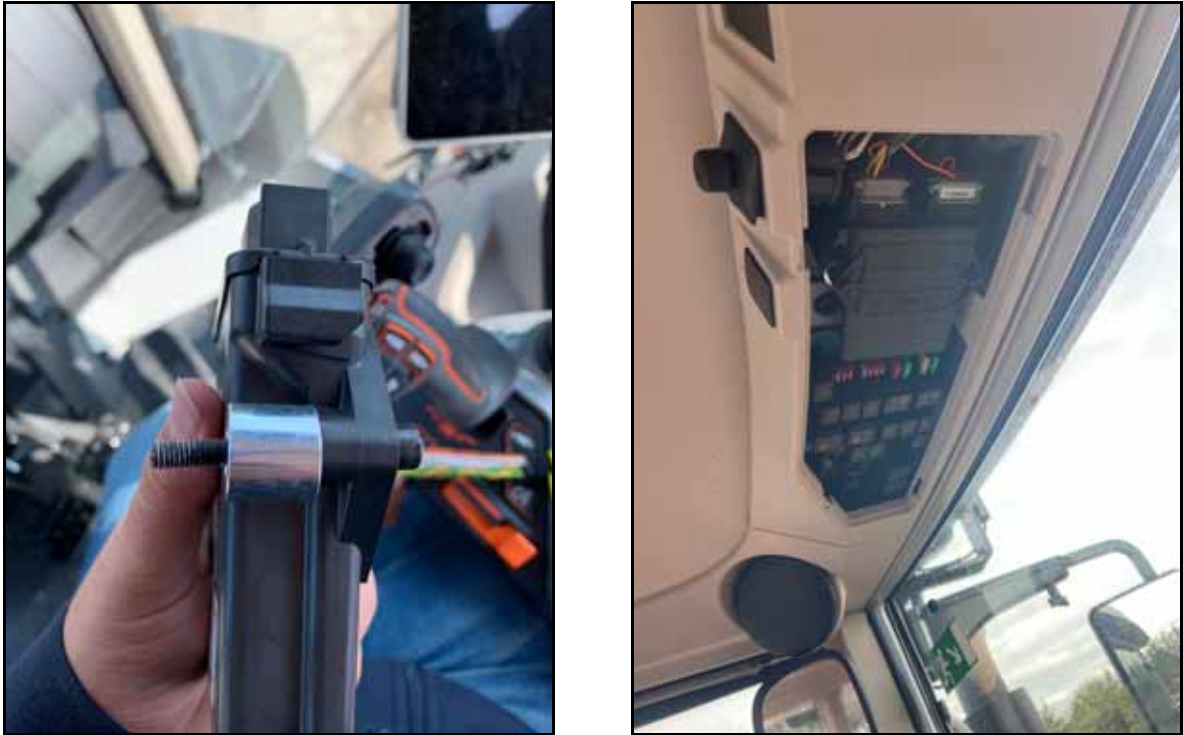
FIGURE 3. Mount the TC1™ ECU
