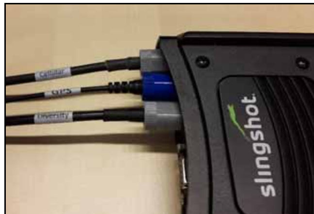
FIGURE 12. Example Slingshot® Field Hub connected with CRx and Viper® 4
