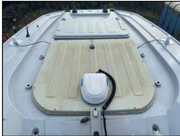
FIGURE 13. GPS Patch Antenna and Two GPRS/UMTS Antennas
