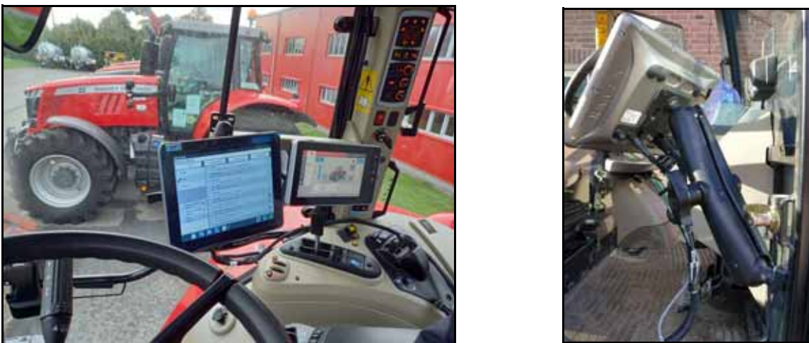
FIGURE 10. CR12™ Mounted in Various Positions
