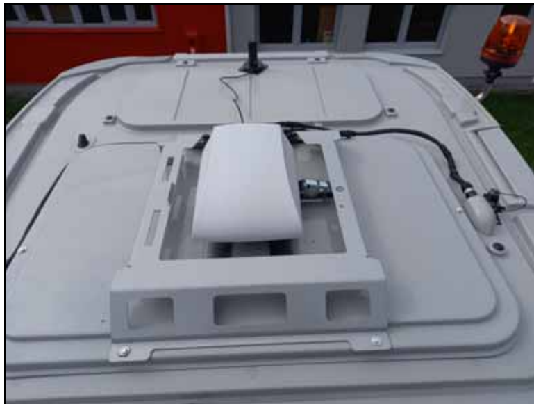
FIGURE 7. RS1™ Mounted and Cable Connected
