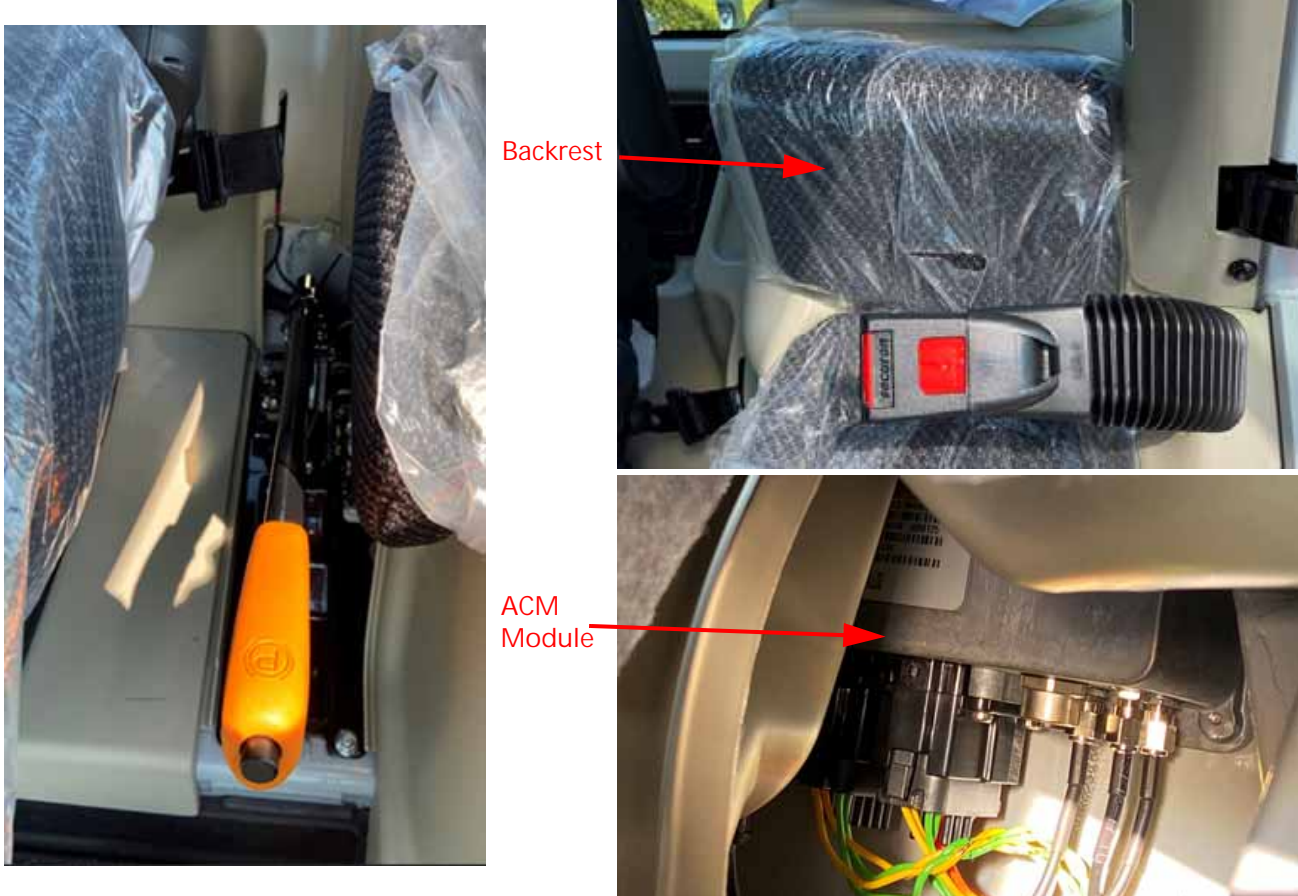
FIGURE 3. ACM Module 5s Location
