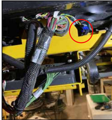
FIGURE 8. Connector with Terminator Removed
