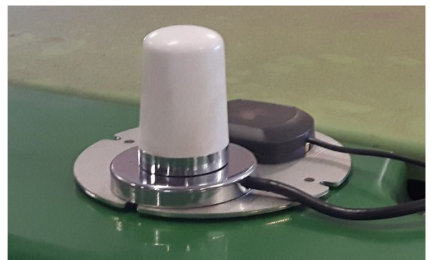
FIGURE 43 GPRS/UMTS-ANTENNA AND GPS PATCH ANTENNA ON A METAL BRACKET
