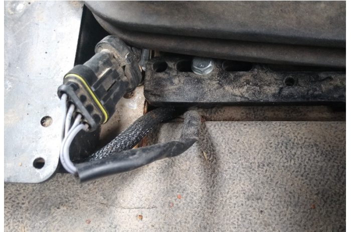
FIGURE 32 EXISTING TRACTOR OPERATOR PRESENC SWITCH CONNECTOR
