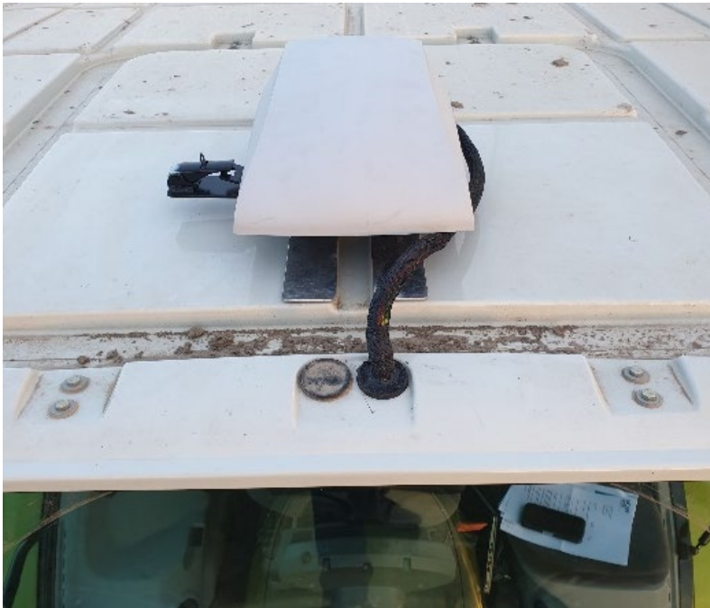
FIGURE 38 RS1 MOUNTED ON TRACTOR
