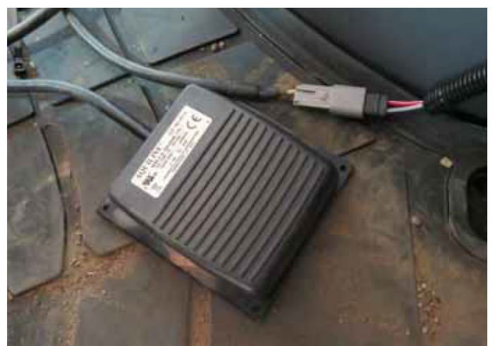
FIGURE 31 RESUME FOOT SWITCH CONNECTION
