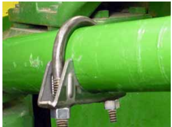
FIGURE 27 EXHAUST CLAMP INSTALLED
