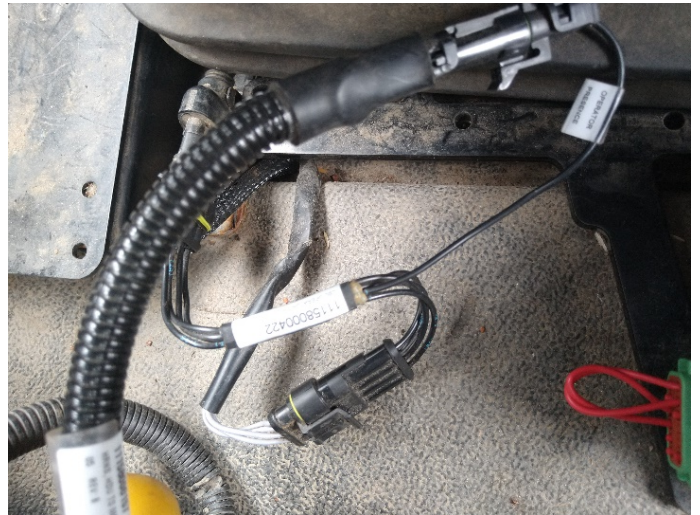
FIGURE 33 OPERATOR PRESENCE SWITCH T-CABLE (115-8000-428) CONNECTION
