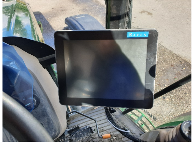
FIGURE 44 CR12 ON A PILLAR
