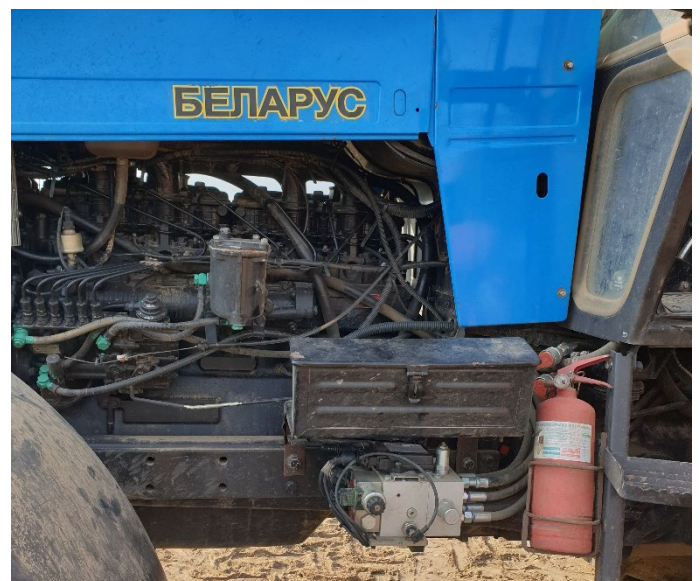
FIGURE 7 MANIFOLD BRACKET WITH A MANIFOLD AND HURAILIC DRIVE UNIT MOUNTED ON MTZ
