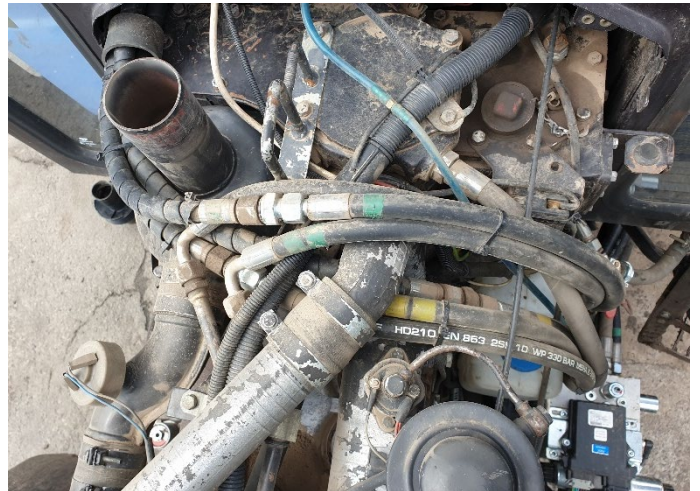
FIGURE 12 LEFT, RIGHT AND PREASURE STEERING HOSES INSTALLED
