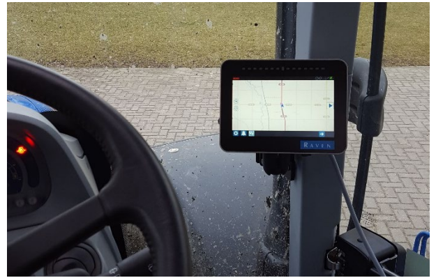
FIGURE 39 CR7 ON A-PILLAR
