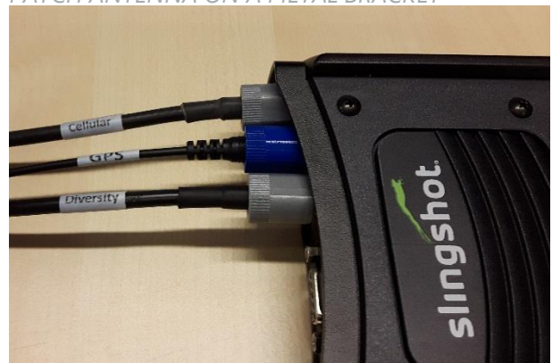
FIGURE 44 ANTENNA CABLES WITH LABELS AND SMA-GRIP SET
