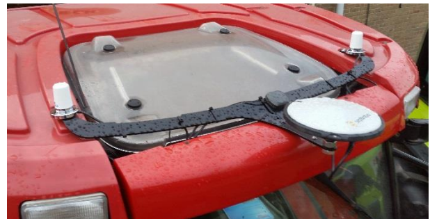
FIGURE 42 CASE NEW HOLLAND WITH GPS-ANTENNA, GPS PATCH ANTENNA AND TWO GPRS/UMTS ANTENNA'S
