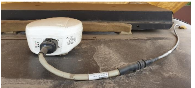
FIGURE 39 600S ANTENNA UNDER SUNROOF
