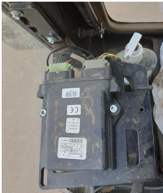
FIGURE 3. SC1/TC1 MOUNTED ON A RIGHT-SIDE PILLAR
