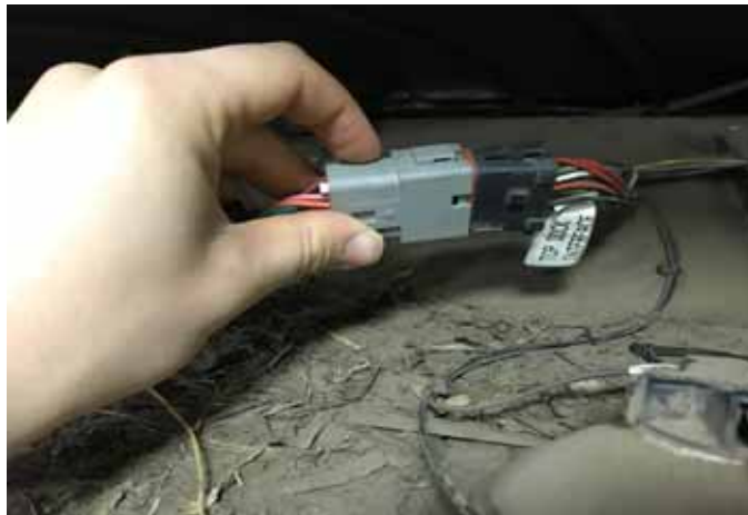
FIGURE 6. Gray Connector Plugged Into Top Dock Interface Connector
