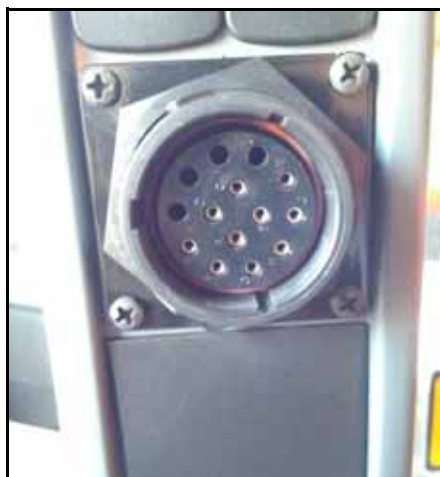
FIGURAS 9. Connector Located on Column of the Tractor
