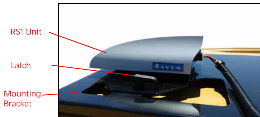
FIGURE 7. Installed RS1 Unit
