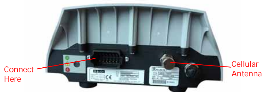
FIGURE 6. Cabling Connection on RS1 Unit
