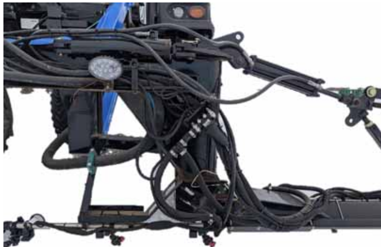
FIGURE 2. Boom Cable Routing - Over Pivot
