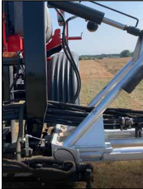
FIGURE 2. Boom Cable Routing - Over Pivot - Pommier Boom
