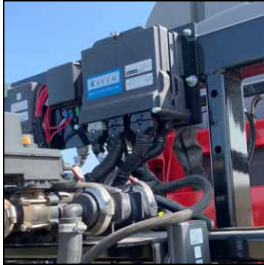
FIGURE 3. RCM - Sprayer Mounting with Raven Autoboam XRT
