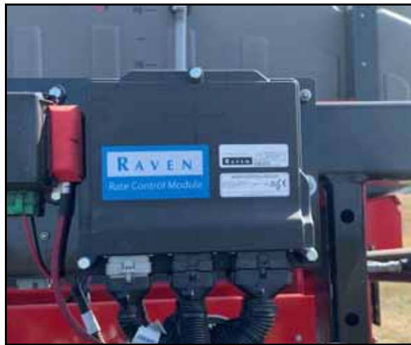
FIGURE 2. RCM - Sprayer Mounting Location and Orientation
