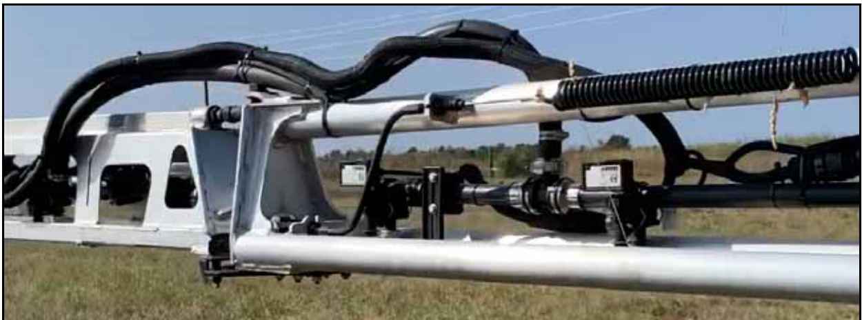
FIGURE 3. Boom Cable Routing - Over Mid Fold Joint
