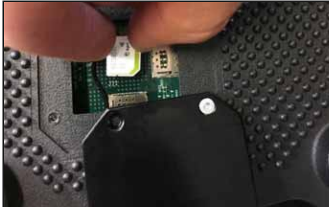
FIGURE 8. SIM Card Inserted in SIM Slot
