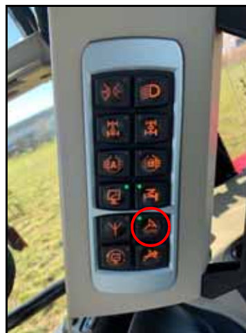
FIGURE 12. Pre-activation Button on C-Pillar
