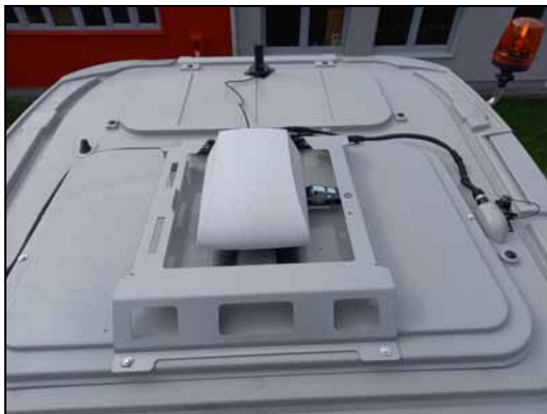
FIGURE 7. RS1 Mounted and Cable Connected
