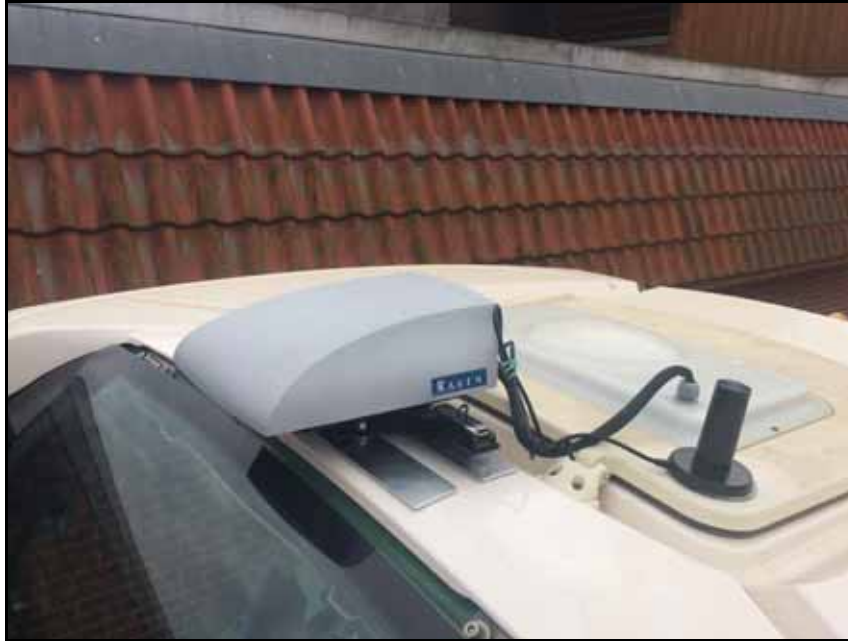
FIGURE 6. Laird Antenna Adhesive Plate
