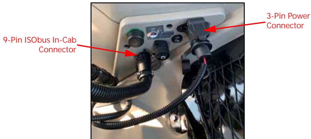
FIGURE 11. ISOBUS and Power Connector
