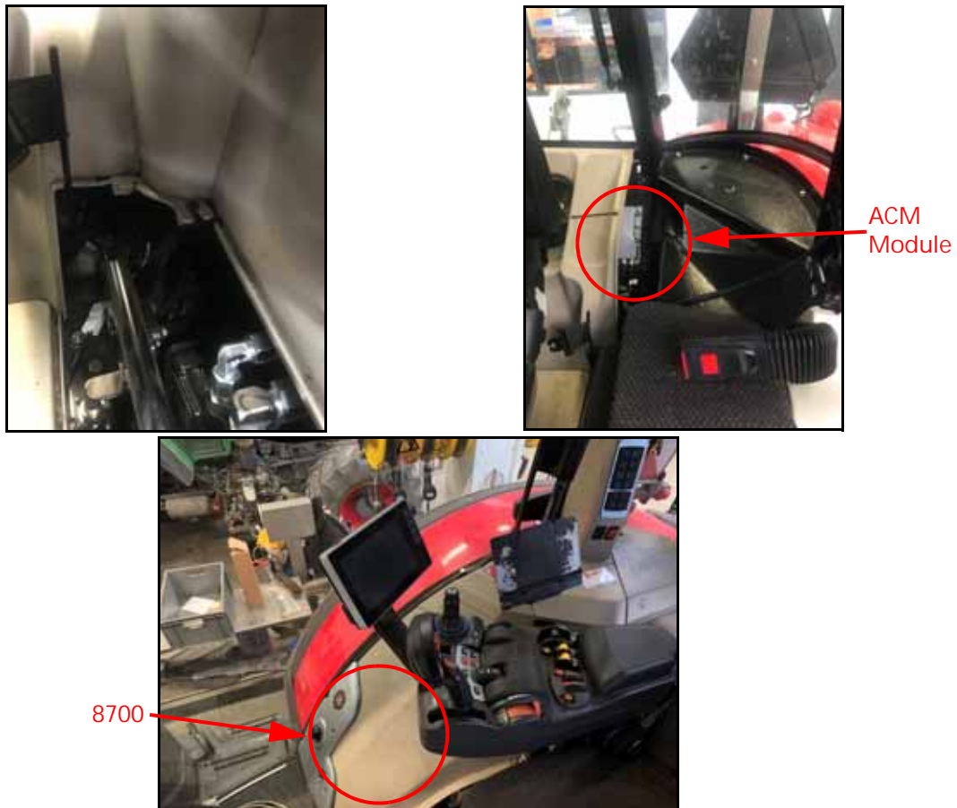
FIGURE 3. Communication Module: 6700, 7700, 8700 Location
