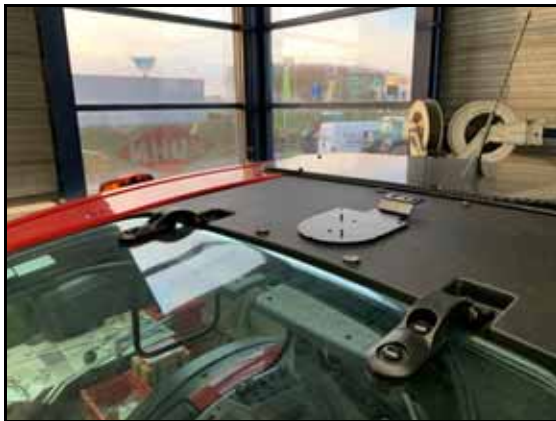
FIGURE 7. 700S Mounting Plate and Antenna
