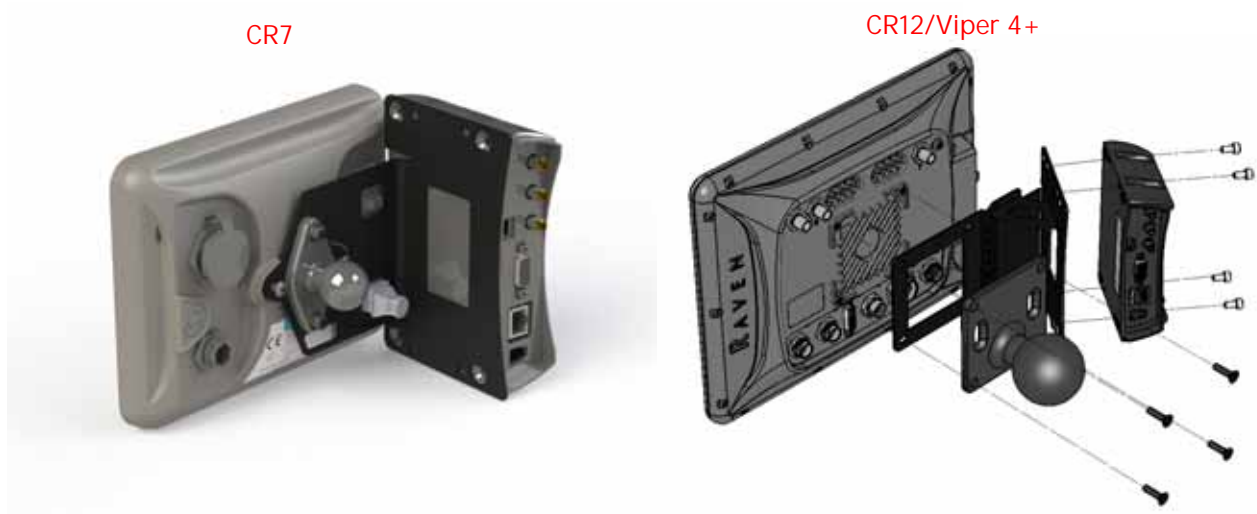
FIGURE 9. Field Hub connected with CRx and Viper 4
