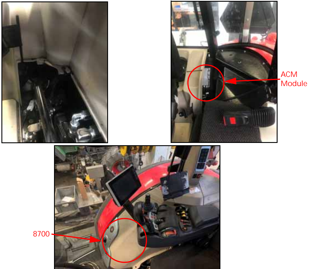
FIGURE 3. Communication Module 6700, 7700, 8700 Location
