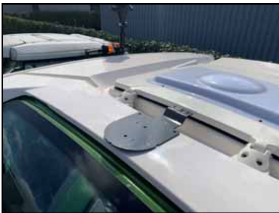
FIGURE 10. 700S Mounting Plate and Antenna
