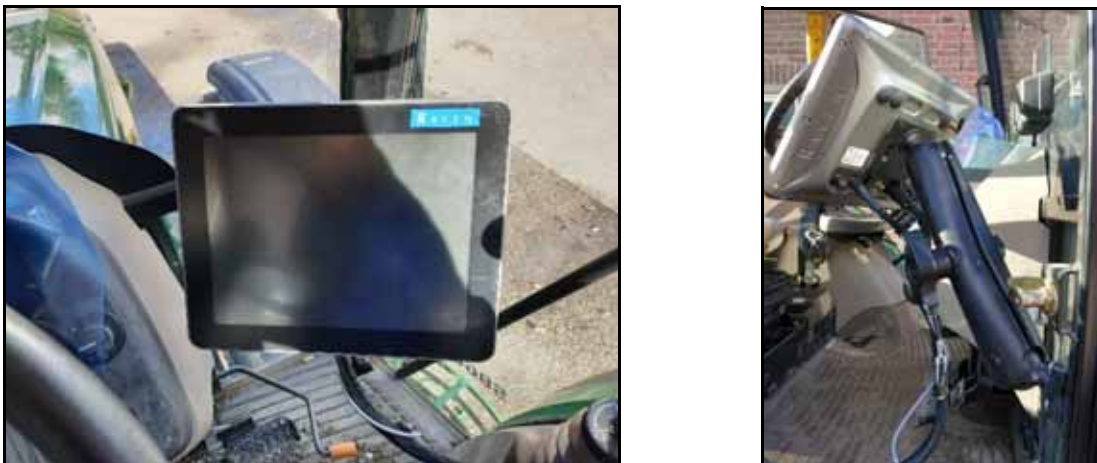
FIGURE 17. CR12 Mounted in Various Positions
