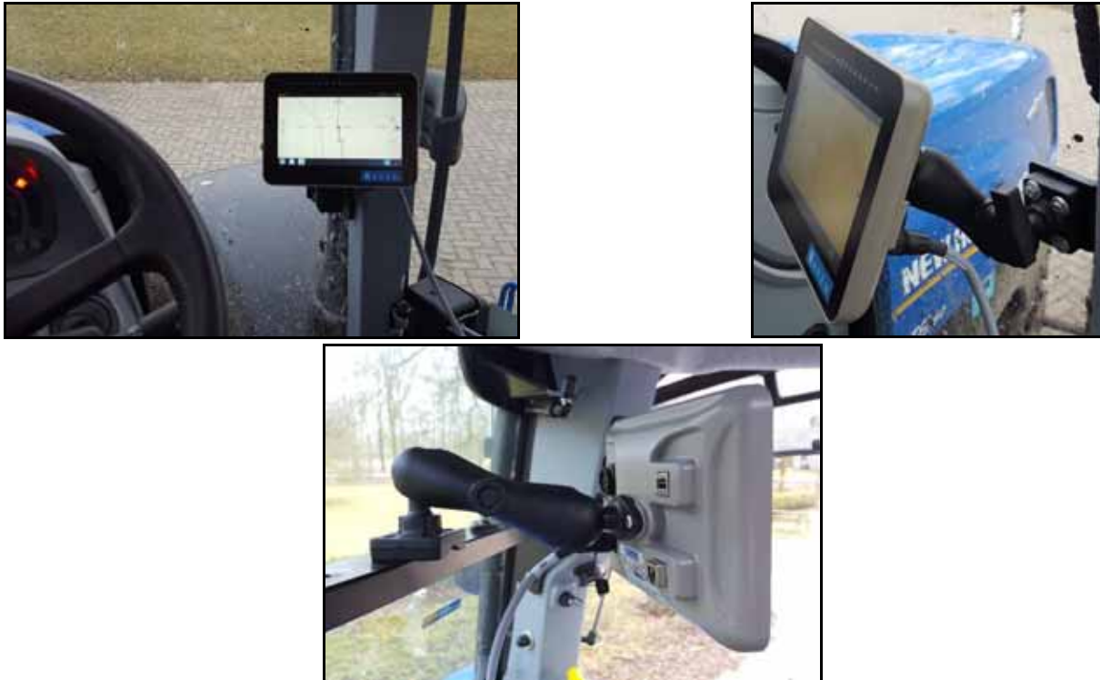
FIGURE 17. CR12 Mounted in Various Positions
