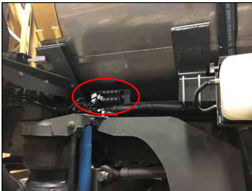
FIGURE 1. Rear CANbus Hub Location
