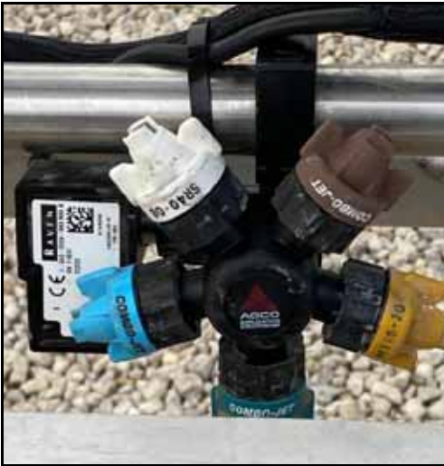
FIGURE 2. Hypro Left-Handed Nozzle Bodies Installed
