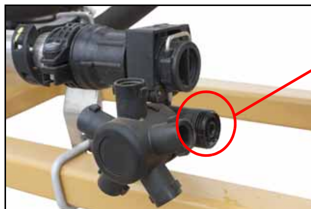
FIGURE 1. Nozzle Body Cap and Diaphragm Removed
