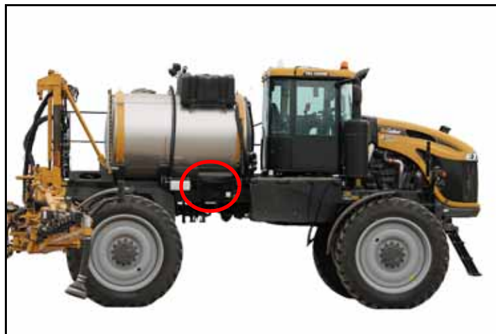
FIGURE 1. Chassis Cable ECU Cabinet Connection
