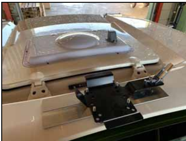
FIGURE 4. Bottom Assembly of RS1 Mount
