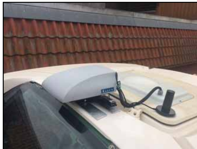
FIGURE 8. Laird Antenna Adhesive Plate
