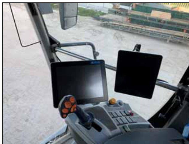
FIGURE 10. Display Mounted on Armrest
