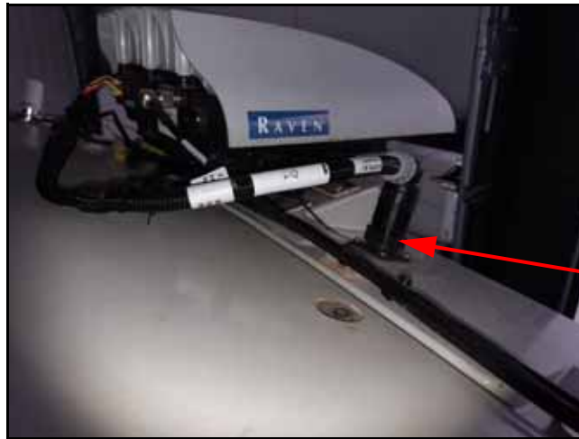
FIGURE 8. Laird Antenna Adhesive Plate
