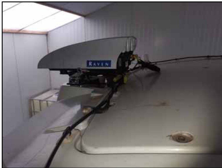
FIGURE 6. RS1 Mounted with Bracket
