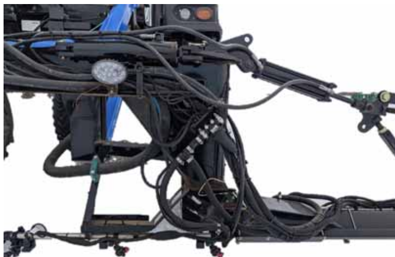
FIGURE 2. Boom Cable Routing - Over Pivot
