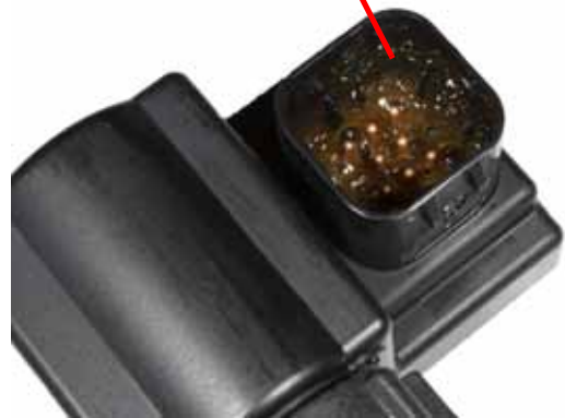
Corrosion Inhibitor Applied
