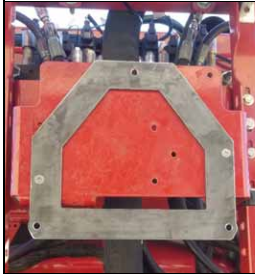
FIGURE 2. RCM - Sprayer Mounting Plate Installed
