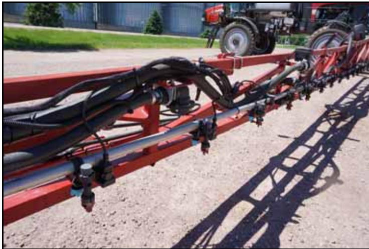
FIGURE 4. Outer Boom Cable Section Installed
