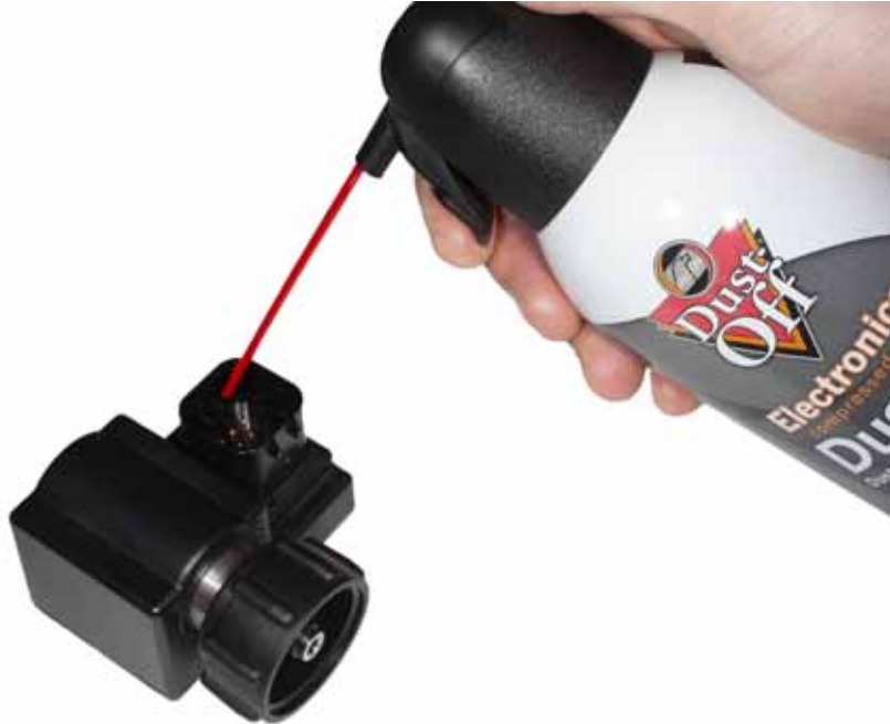
FIGURE 3. Compressed Air Applied for Drying
