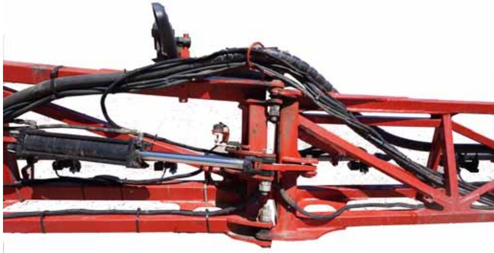
FIGURE 3. Boom Cable Routing - Over Mid Fold Joint
