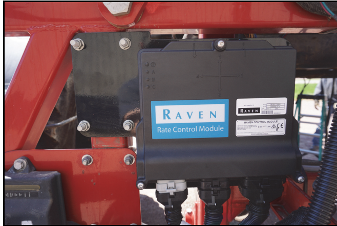
FIGURE 4. RCM - Sprayer Secured to Mounting Plate
