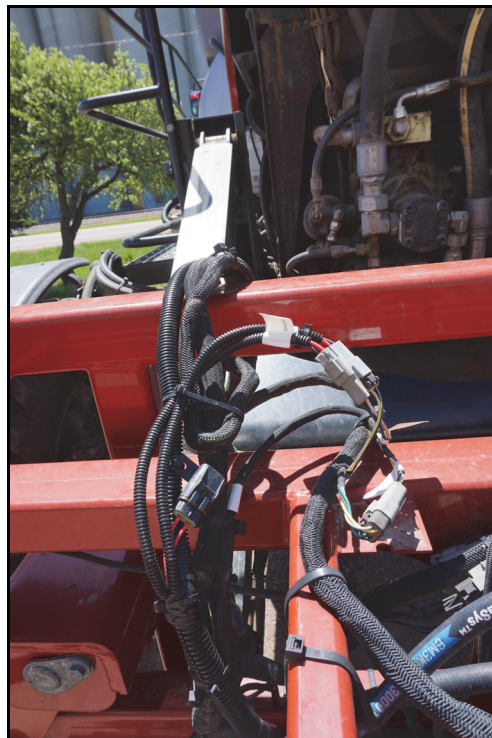
FIGURE 6. RCM - Sprayer Power/Ground and ISObus Connections
