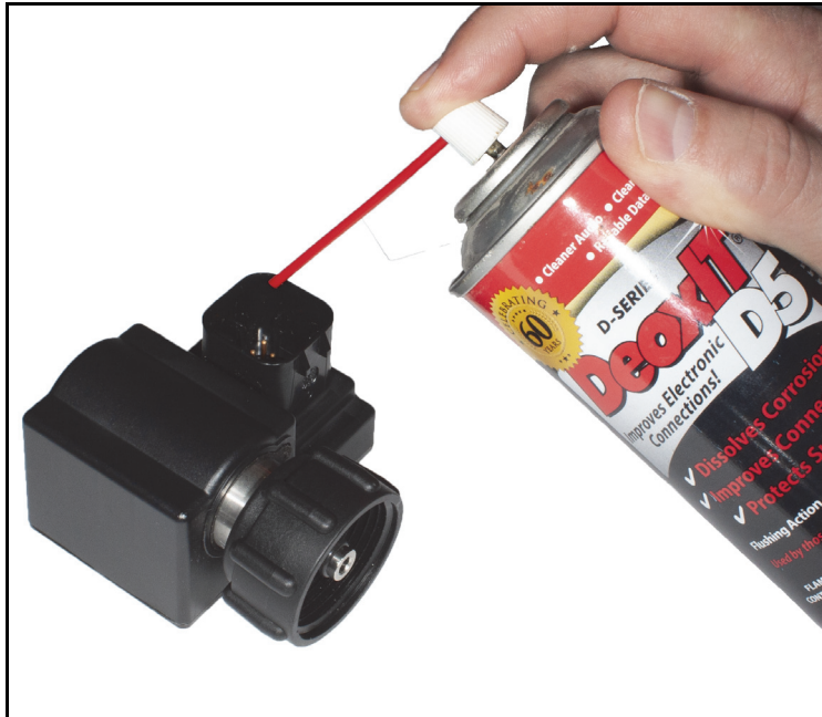
FIGURE 1. Deoxidizing Agent Applied to Connection
