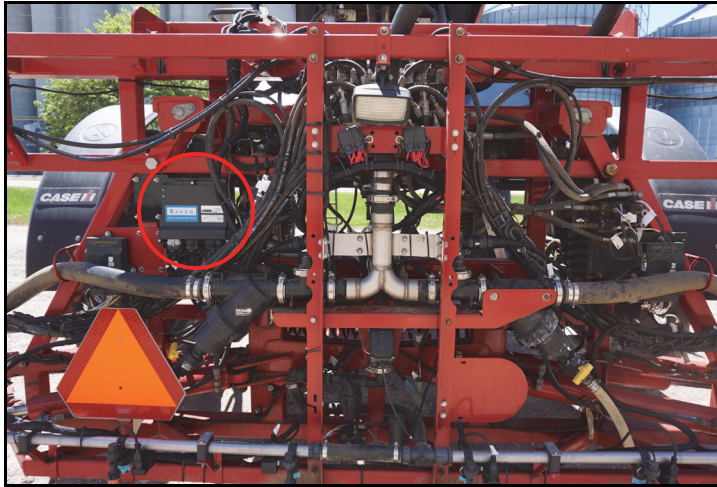
FIGURE 2. RCM - Sprayer Installation Location
