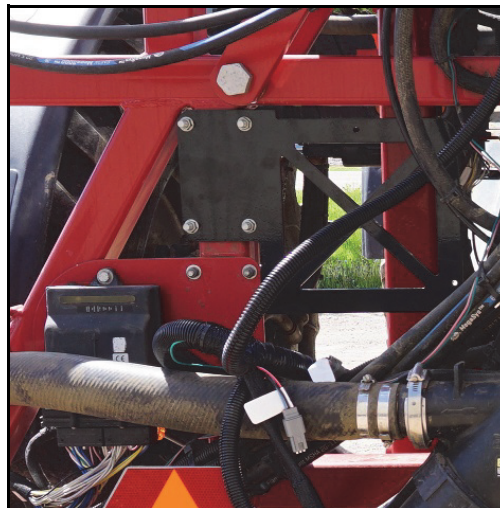
FIGURE 3. RCM - Sprayer Mounting Plate Installed
