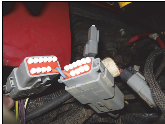
FIGURE 15. Fence Row Adapter Cable Installed
