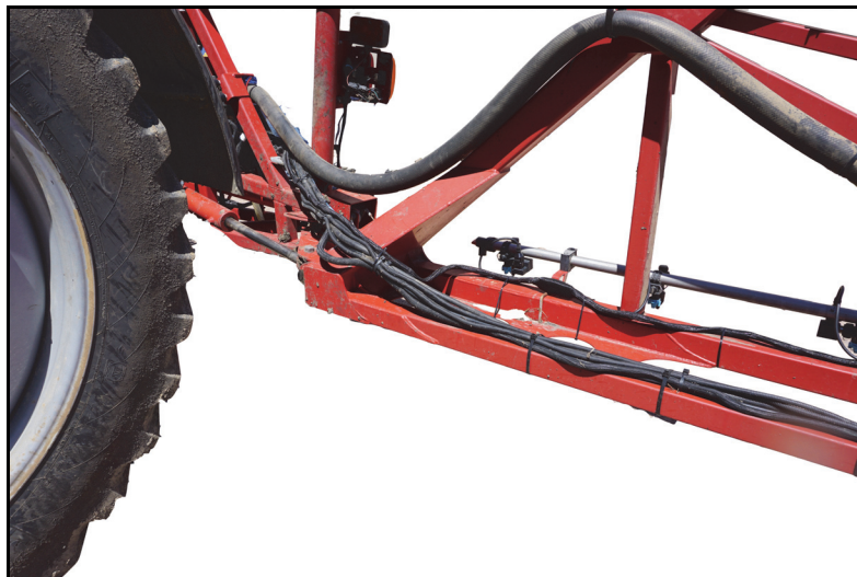
FIGURE 2. Boom Cable Routing - Over Pivot
