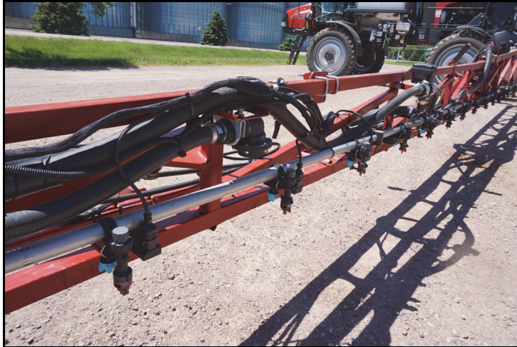
FIGURE 4. Outer Boom Cable Section Installed
