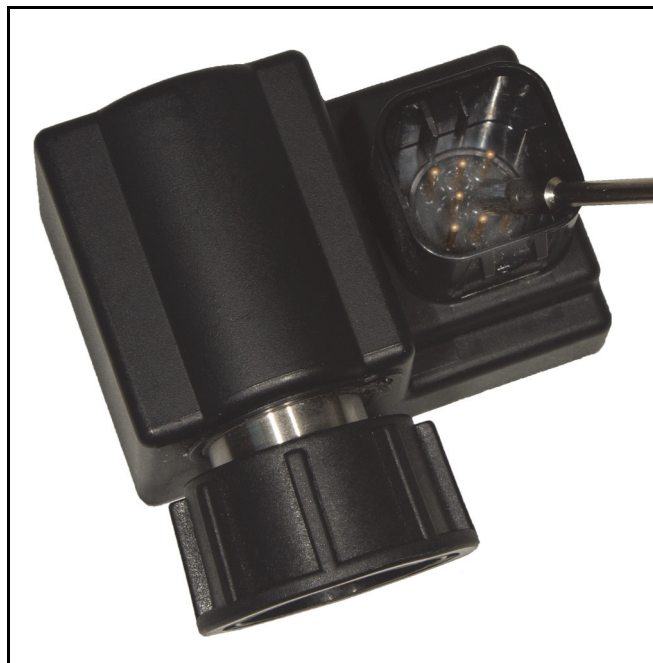
FIGURE 2. Connection Contact Cleaning
