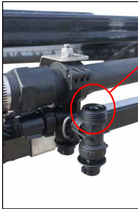
FIGURE 1. Nozzle Body Cap and Diaphragm Removed
