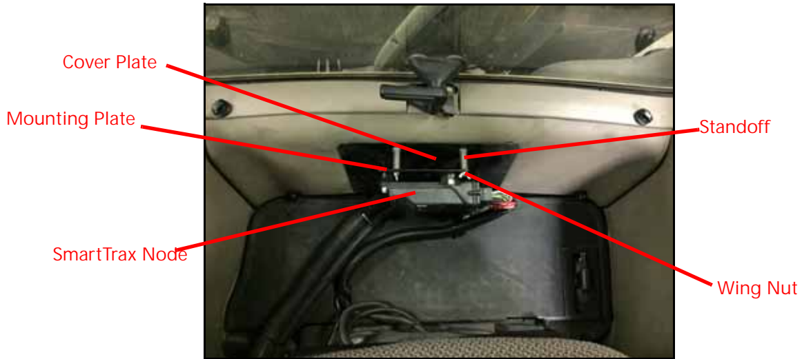
FIGURE 2. SmarTrax Node on Mounting Plate
