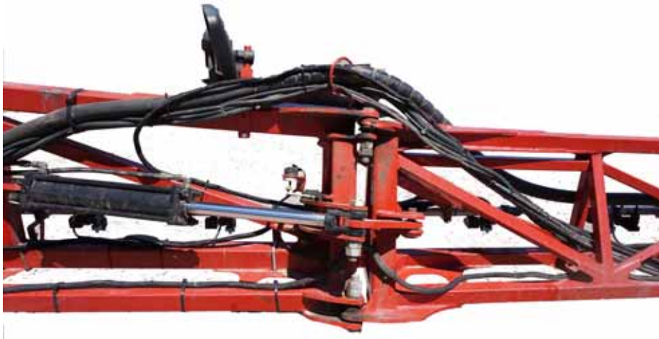
FIGURE 3. Boom Cable Routing - Over Mid Fold Joint
