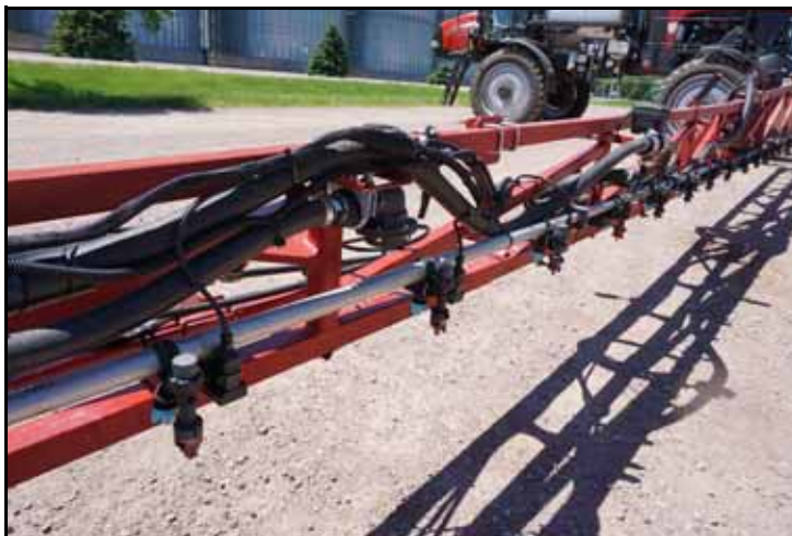
FIGURE 4. Outer Boom Cable Section Installed
