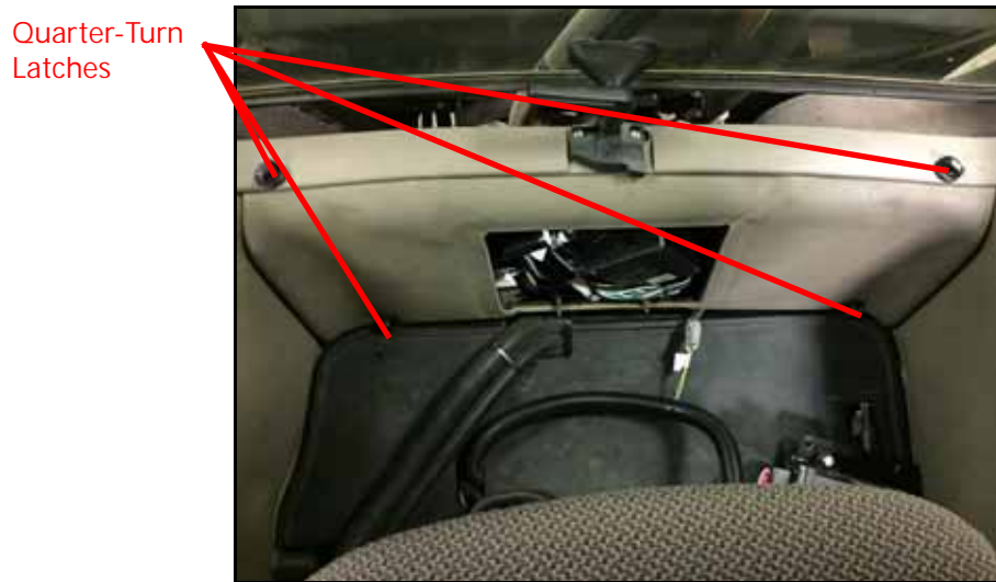
FIGURE 3. Quarter-Turn Latches for Back Panel
