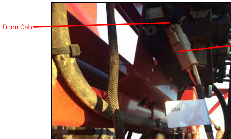
FIGURE 8. Four-Pin from RCM- Sprayer Harness
