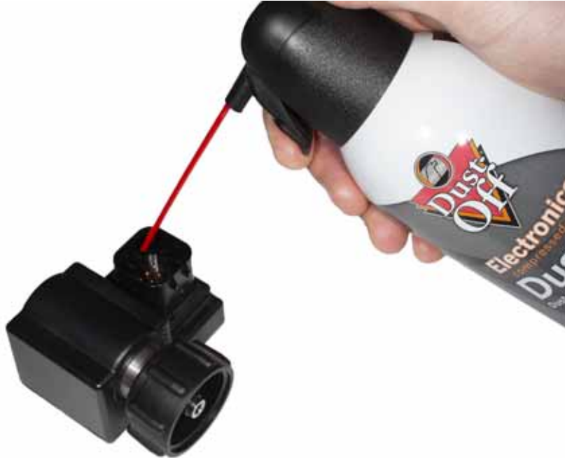
FIGURE 3. Compressed Air Applied for Drying
