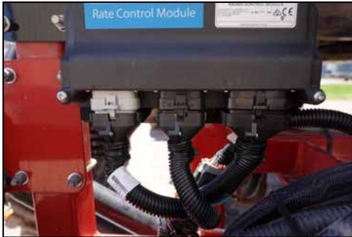
FIGURE 5. RCM - Sprayer Connections
