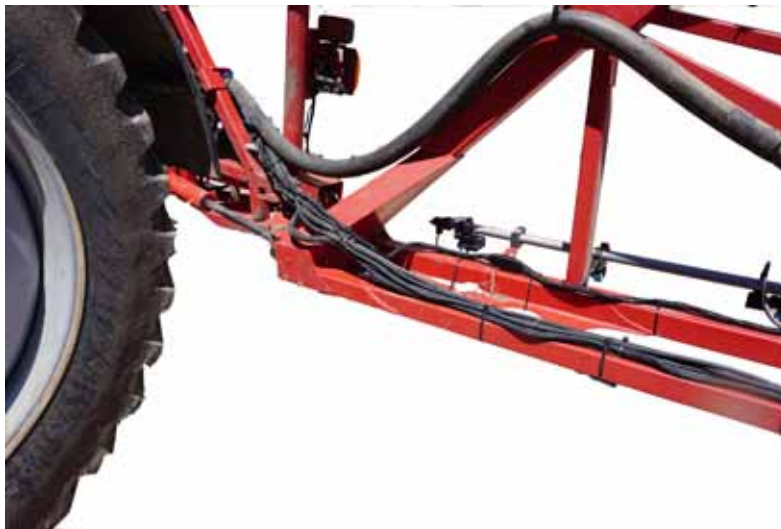
FIGURE 2. Boom Cable Routing - Over Pivot
