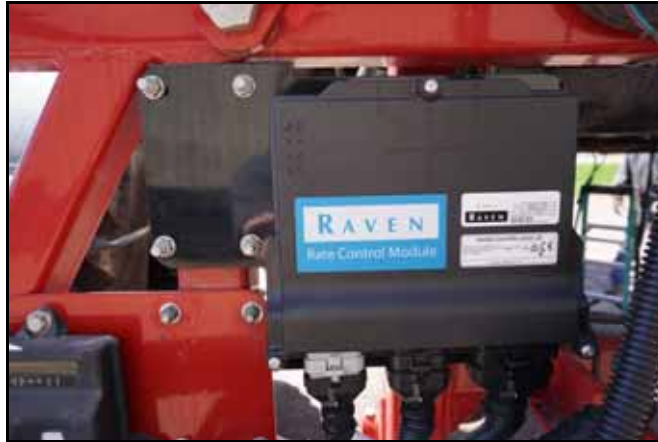
FIGURE 4. RCM - Sprayer Secured to Mounting Plate
