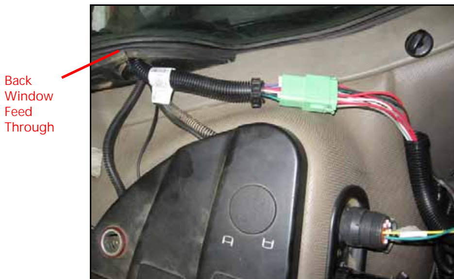
FIGURE 5. Feed Through in Back Window
