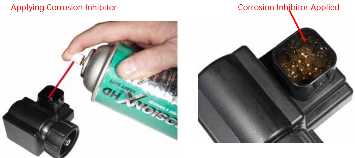
FIGURE 4. Corrosion Inhibitor Check
