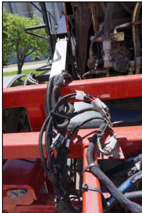
FIGURE 6. RCM - Sprayer Power/Ground and ISObus Connections
