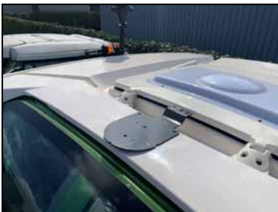
FIGURE 2. 700S Mounting Plate and Antenna
