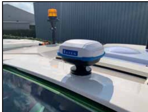
FIGURE 2. 700S Mounting Plate and Antenna
