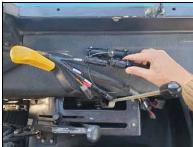
FIGURE 6. Cable Connected to 9-Pin ISO Connector
