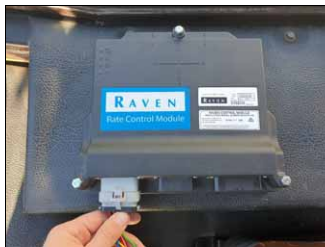
FIGURE 4. RCM Power Cable Connected
