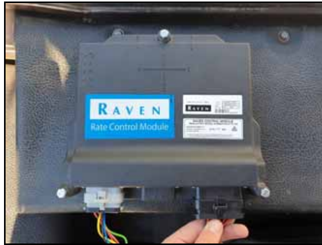
FIGURE 5. RCM to ARAG Cable Connected
