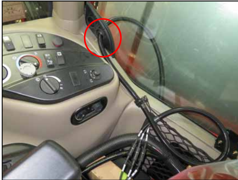
FIGURE 12. Cab Access Point
