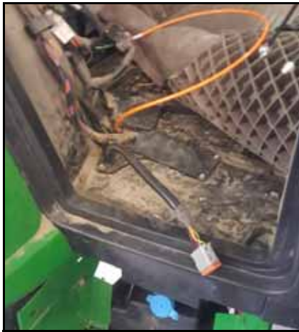
FIGURE 9. Cable Routed through Cab Floor
