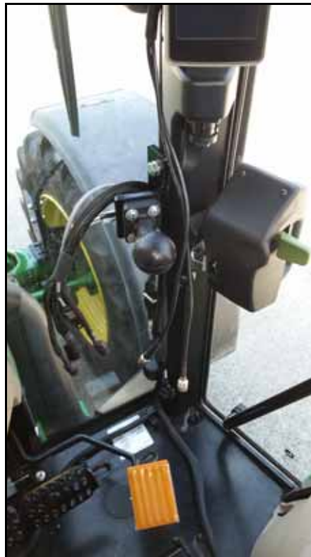
FIGURE 11. Field Computer Harness from Floor to A-Pillar
