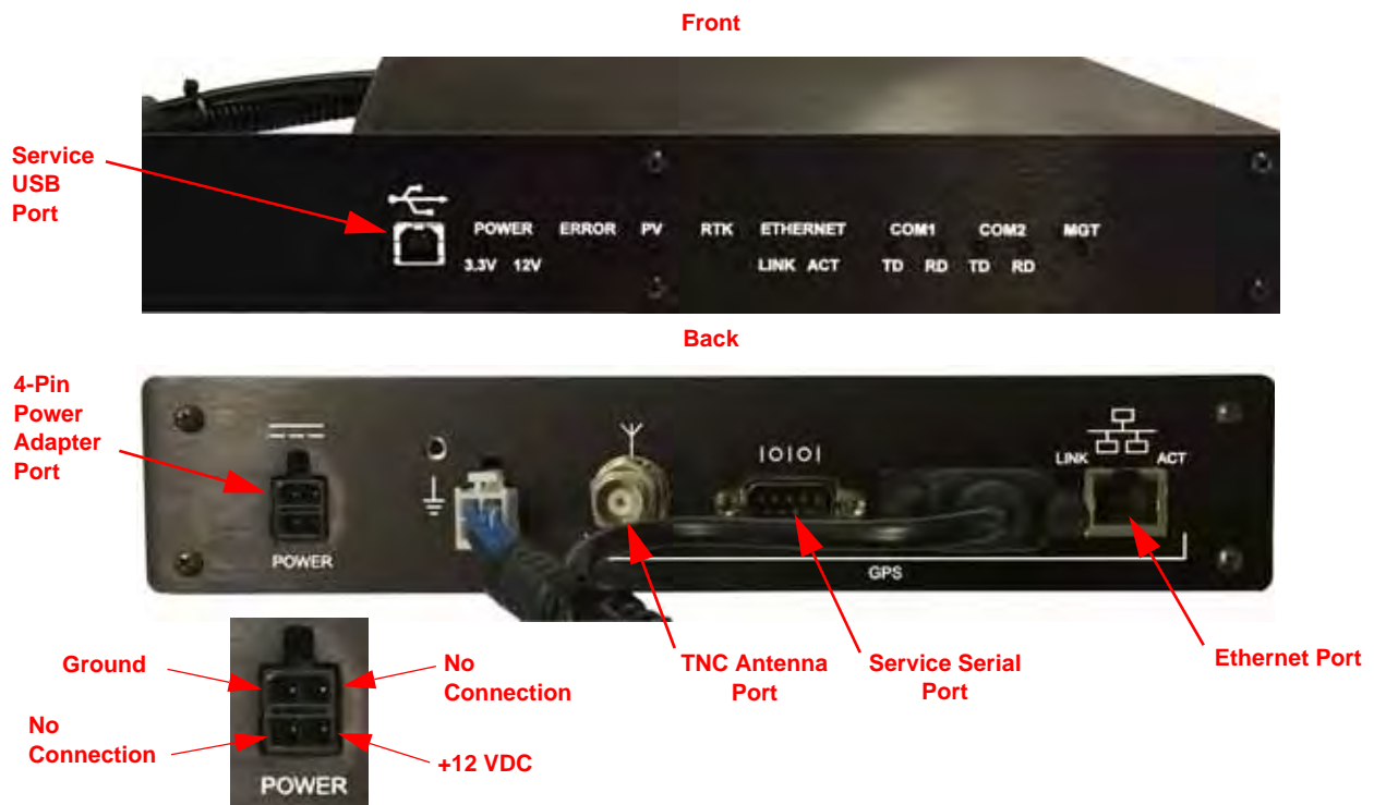
FIGURE 1. Base Station 2.0 Connectors
