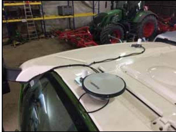
FIGURE 18. GPS Patch Antenna and Two GPRS/UMTS Antennas
