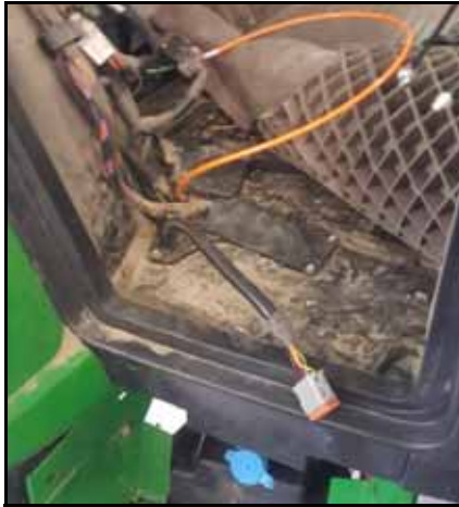
FIGURE 9. Cable Routed through Cab Floor
