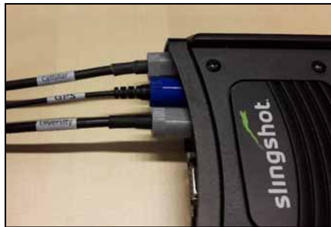
FIGURE 15. Field Hub connected with CRx and Viper 4
