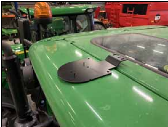
FIGURE 12. 700S Mounting Plate and Antenna
