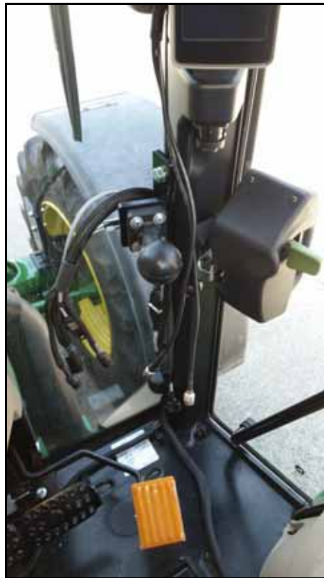
FIGURE 9. Field Computer Harness from Floor to A-Pillar
