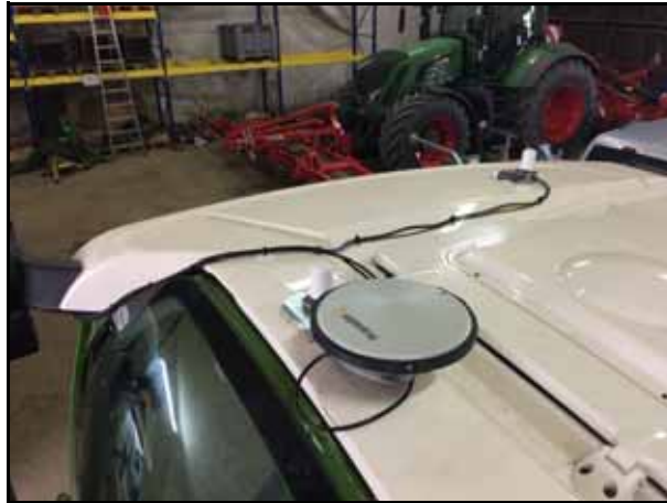
FIGURE 16. GPS Patch Antenna and Two GPRS/UMTS Antennas
