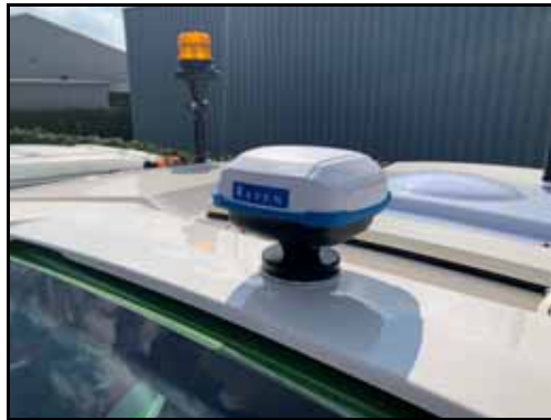
FIGURE 12. 700S Mounting Plate and Antenna
