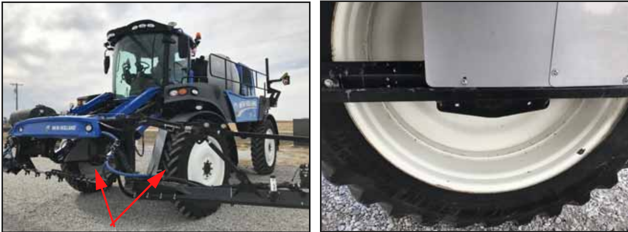
FIGURE 7. Removed Wheel Motor Covers
