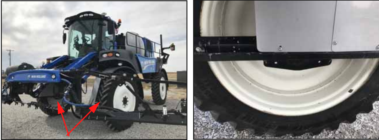
FIGURE 7. Removed Wheel Motor Covers
