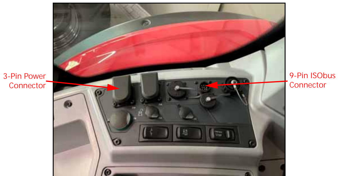
FIGURE 15. ISOBUS and Power Connector
