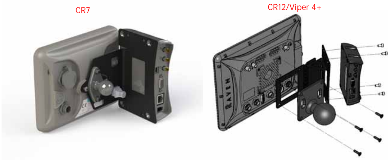
FIGURE 10. Field Hub connected with CRx and Viper 4
