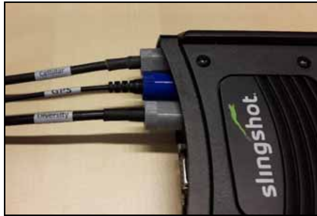
FIGURE 10. Field Hub connected with CRx and Viper 4
