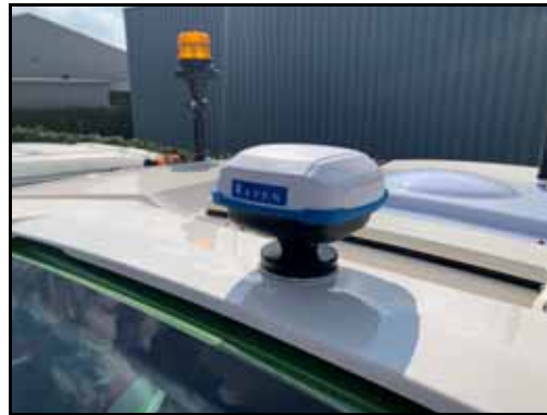
FIGURE 7. 700S Mounting Plate and Antenna
