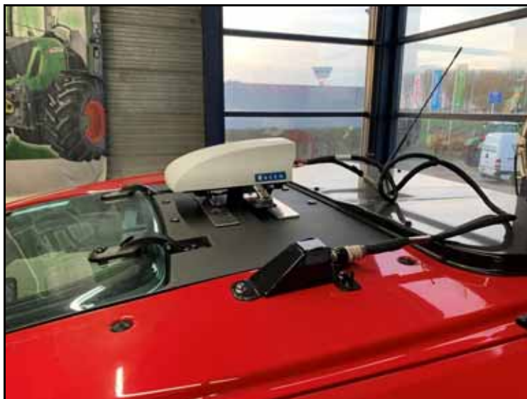
FIGURE 4. RS1 Mounted and Cable Connected
