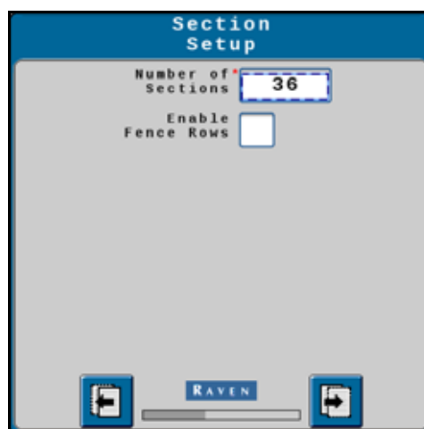
FIGURE 1. Section Setup - Number of Sections
