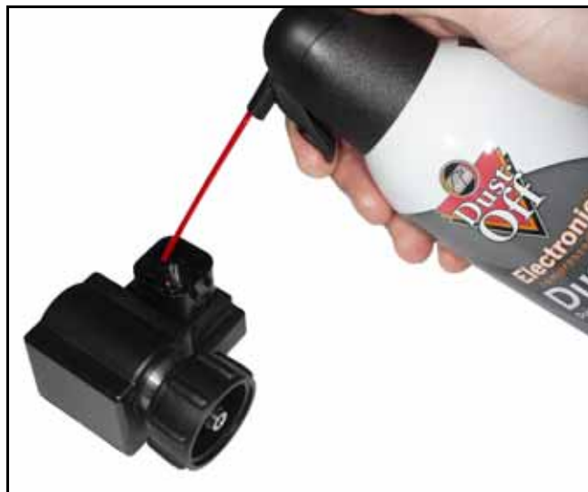
FIGURE 3. Electronics Duster Used on NCV
