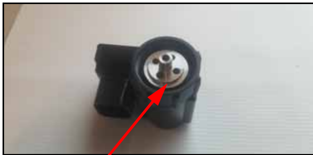
FIGURE 1. Valve Face O-Ring and Nozzle Control Valve Installed
