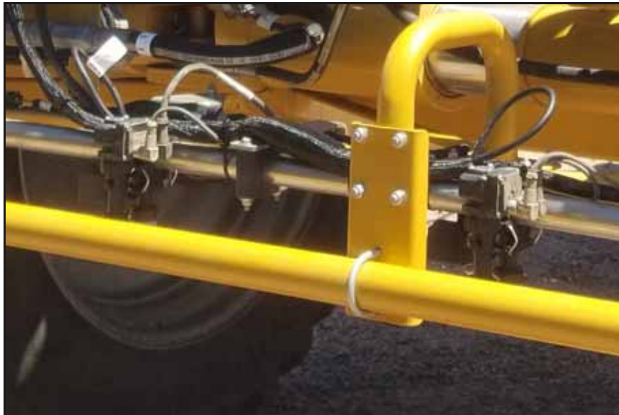
FIGURE 9. Completed Wilger Assembly
