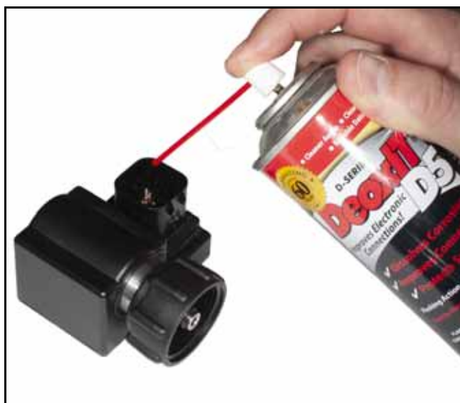
FIGURE 1. DeoxIT D5 Applied to Hawkeye® 2 NCV
