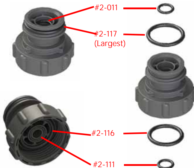
FIGURE 7. ProStop-E Adapter O-Ring Installation
