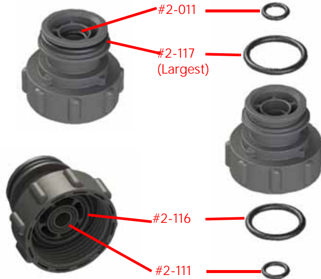
FIGURE 7. ProStop-E Adapter O-Ring Installation
