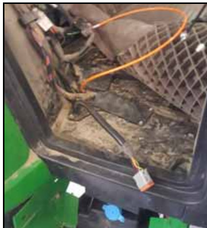
FIGURE 10. Cable Routed through Cab Floor
