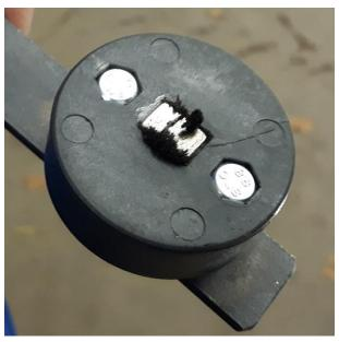
FIGURE 27 DIRTY WHEEL ANGLE SENSOR MAGNET.
