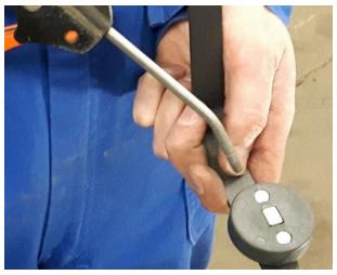
FIGURE 28 CLEANING WHEEL ANGLE SENSOR.
