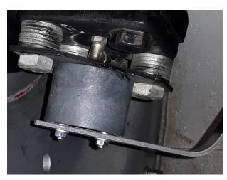
FIGURE 30 CORRECT MOUNTED WHEEL ANGLE SENSOR
