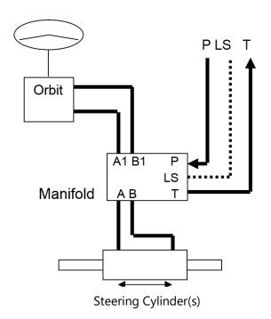
FIGURE 6 LOAD SENSE CONNECTING CIRCUIT
