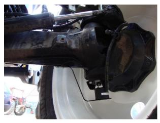
FIGURE 19 STEERING ANGLE SENSOR ON NEW HOLLAND.
