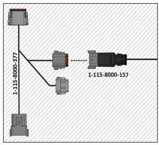
FIGURE 33 CONNECTED 115-8000-157 TO THE 115-8000-377
