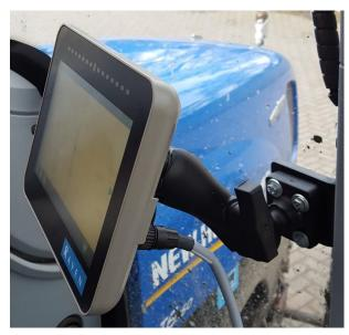
FIGURE 49 RAM-C BALL ATTACHEMENT
