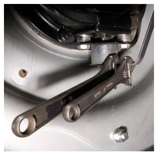
FIGURE 24 BEND THE STRIP WITH THE HELP OF TWO AJUSTABLE WRENCHES.
