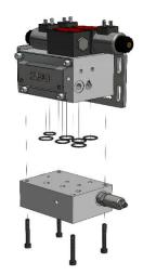
FIGURE 10 ADD-ON PART OF THE OPEN CENTER MANIFOLD
