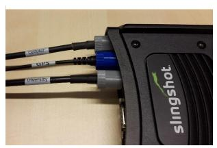
FIGURE 47 ANTENNA CABLES WITH LABELS AND SMA-GRIP SET.
