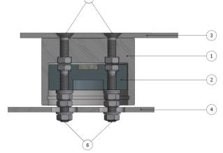
FIGURE 17 SCHEMATIC DRAWING OF WHEEL ANGLE SENSOR WHEN MOUNTED
