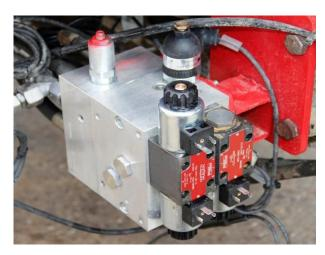
FIGURE 9 OPEN CENTER MANIFOLD
