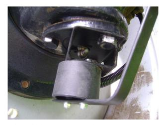
FIGURE 20 STUB AXLE WITH GREASE NIPPLE.
