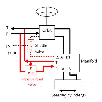
FIGURE 13 PRESSURE RELIEF VALVE CONNECTION.
