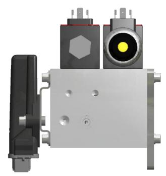
FIGURE 14 SIDE VIEW OF THE HYDRAULIC DRIVE UNIT TO THE MANIFOLD
