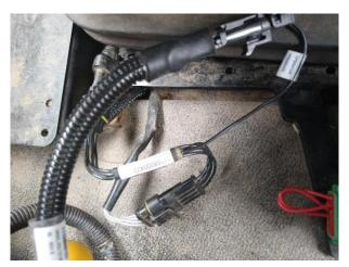
FIGURE 38 OPERATOR PRESENCE SWITCH T-CABLE (115-8000-428) CONNECTION
