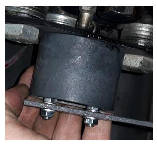
FIGURE 29 CENTRE AND FRICTION CHECK OF WHEEL ANGLE SENSOR.
