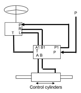
FIGURE 11 OPEN CENTER CONNECTION CIRCUIT
