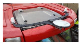
FIGURE 45 CASE NEW HOLLAND WITH GPS-ANTENNA, GPS PATCH ANTENNA AND TWO GPRS/UMTS ANTENNA'S
