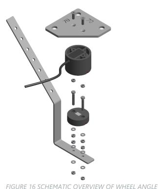
SENSOR WITH MOUNTING BRACKET AND STRIP
