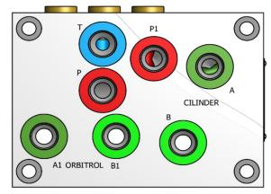
FIGURE 12 CONNECTIONS OF THE HYDRAULIC OPEN CENTER MANIFOLD
