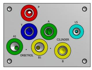
FIGURE 7 CONNECTIONS FOR THE HYDRAULIC LOAD SENSE MANIFOLD
