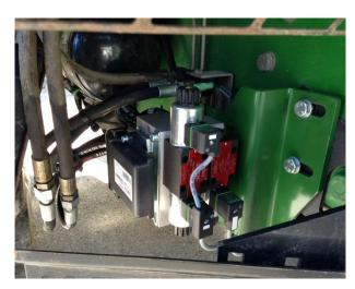
FIGURE 5 MOUNTED MANIFOLD AND STEERING CONTROLLER
