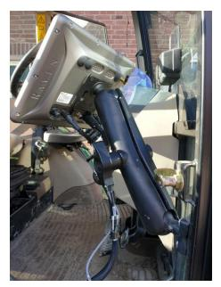
FIGURE 52 RAM D BALL ATTACHMENT ON PILAR
