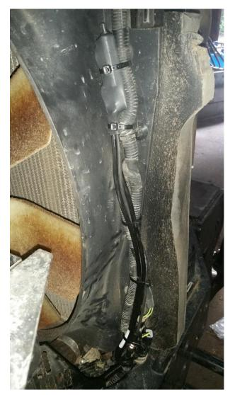
FIGURE 15 SPY CABLE MOUNTED ON A CNH TRACTOR
