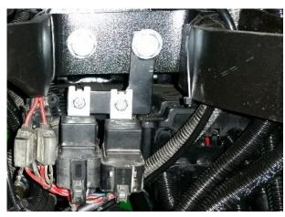
FIGURE 2 CORRECT MOUNTED RELAYS AND FUSES
