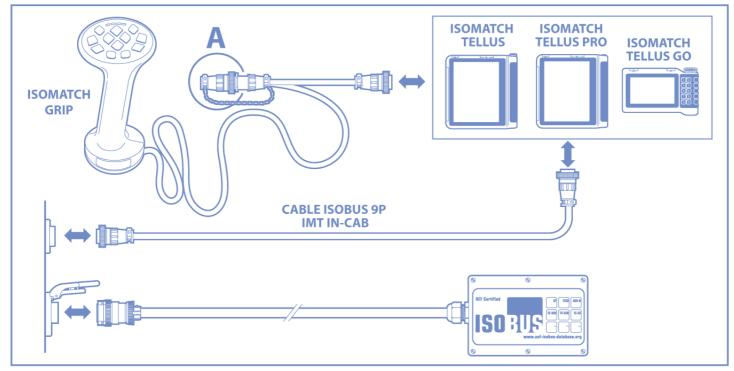
**Detail A:** Connector can be connected to other 'incab devices'. Always use the protective cap when not connected to another device.
