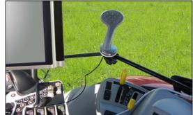
Then connect the IsoMatch Grip to the ISOBUS incab connector.
