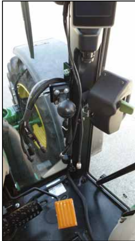
FIGURE 9. Field Computer Harness from Floor to A-Pillar
