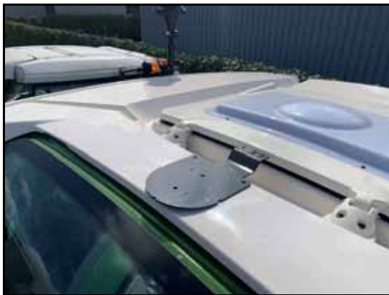
FIGURE 12. 700S Mounting Plate and Antenna
