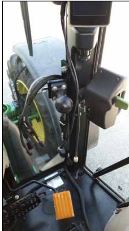
FIGURE 9. Field Computer Harness from Floor to A-Pillar
