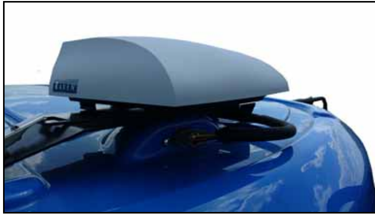
FIGURE 4. Completed Cab Top Installation
