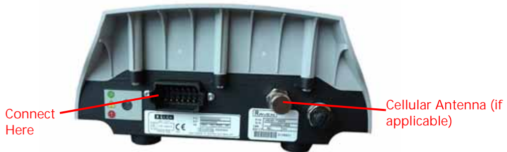
FIGURE 3. Cabling Connection on RS1 Unit
