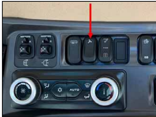
FIGURE 8. Headliner Roothing Switch
