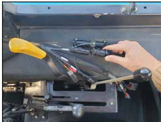
FIGURE 7. Cable Connected to 9-Pin ISO Connector
