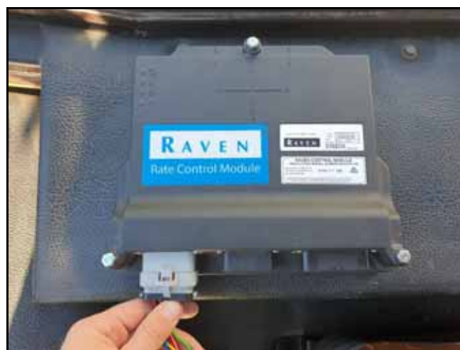
FIGURE 5. RCM Power Cable Connected
