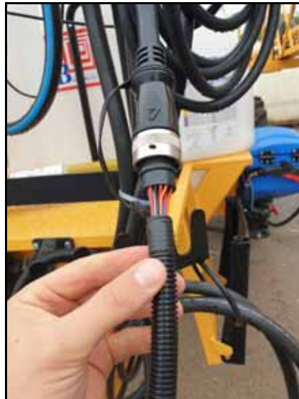
FIGURE 8. RCM to ARAG Product Cable Connected to ARAG Product Cable
