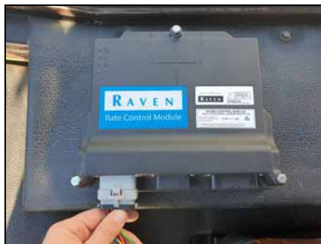
FIGURE 4. RCM Power Cable Connected
