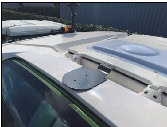
FIGURE 13. 700S Mounting Plate and Antenna
