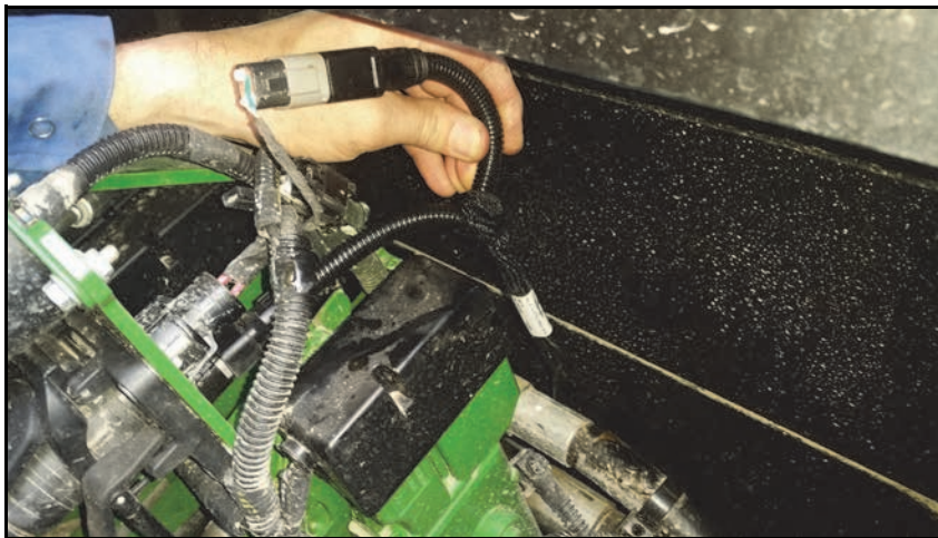
FIGURE 8. Y-Cable Mounted Between Existing ISOBUS Cable
