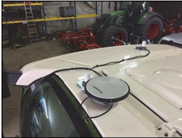
FIGURE 17. GPS Patch Antenna and Two GPRS/UMTS Antennas
