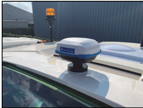
FIGURE 13. 700S Mounting Plate and Antenna
