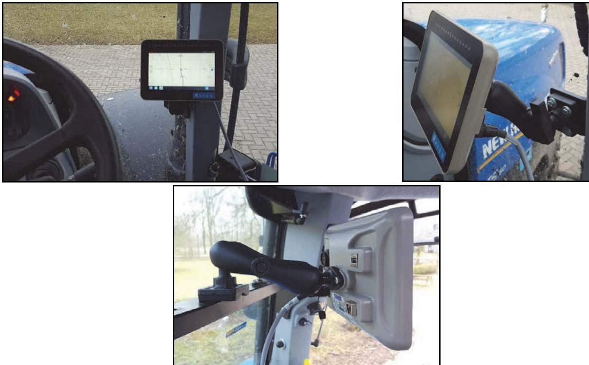
FIGURE 20. CR12 Mounted in Various Positions
