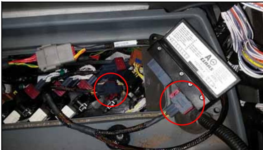
8. Use the opening on the right side of the cab to guide the antenna cables to the front of the cab.
