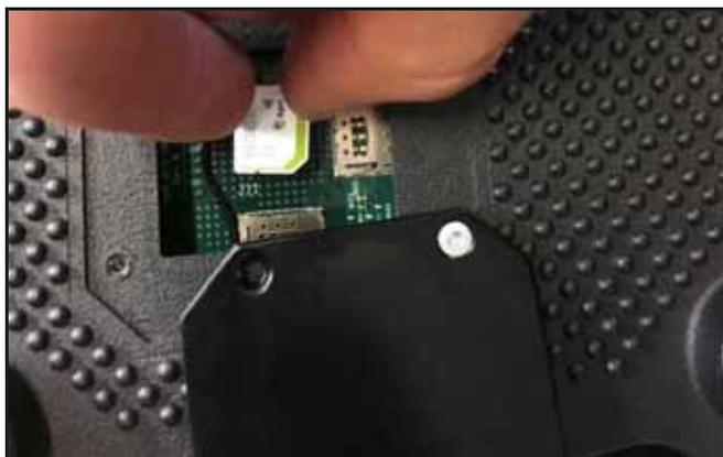
**NOTE:** The SIM card must be inserted into the J11 slot or the RS1 will not receive any GPS signal.
