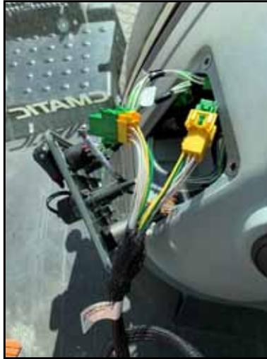
5. Route the 115-4010-181 cable and the 115-4010-186 cable to the roof gland connector and connect the cables to the roof gland.
