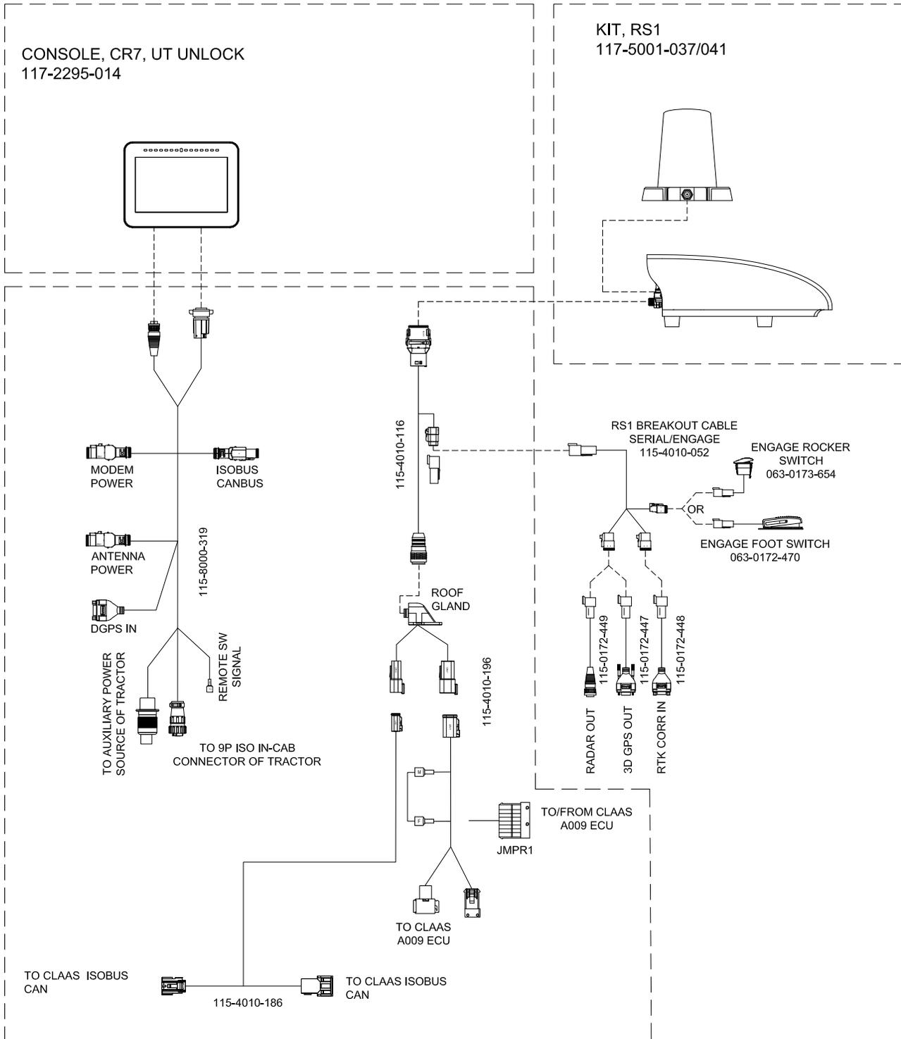
FIGURE 20. Claas ATP CR12 & RS1 System Drawing (P/N 054-5036-037 Rev. A)
