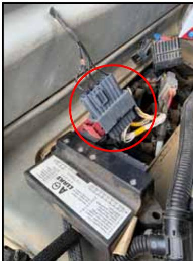
7. Disconnect the 6-pin connector from the ATP2 module and mount the 115-4010-195 cable between the original connector and the ATP2 module.
