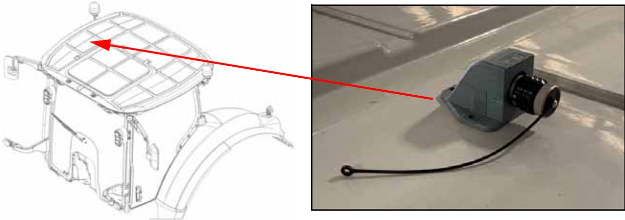
NOTE: Ensure the RS1 cable is long enough to reach the roof gland or mount the roof gland within the length of the RS1 cable.
