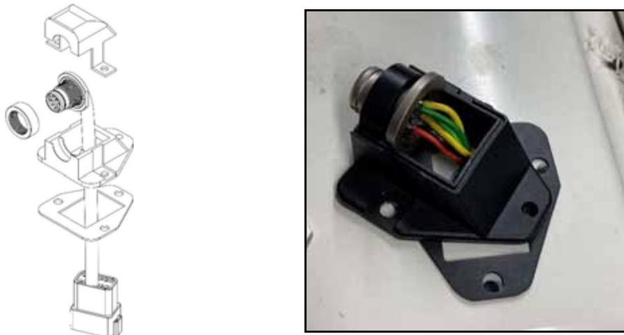
14. Mount the roof gland with the supplied self-drilling screws.
