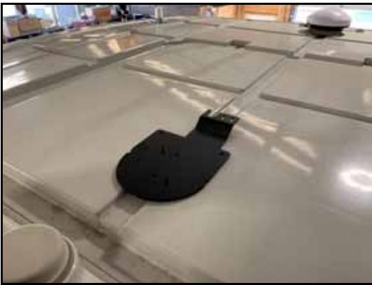
FIGURE 13. 700S Mounting Plate and Antenna
